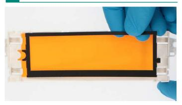
Position the frame supplied with the kit on the backlight diffuser underneath the display.
