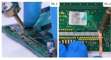
De-solder the original display with a hot air de-soldering iron (Pic. 1). Clean with a solder wick and a soldering iron with chisel tip to remove any excess tin (Pic. 2).
