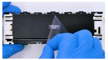
Put back the module in the rear cover, making sure not to damage the FPC. Then, peel off the front film.
