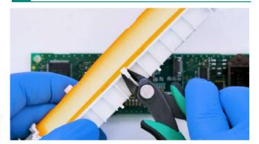
With a flush cutter, **cut off the central clip of the plastic base** of the display and any other plastic part positioned by the new FPC, as it may damage it when re-assembling.
