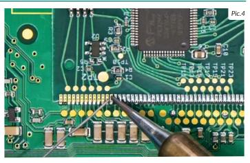
Position the small PCB leaving 1mm gap, as in picture 3, and solder each pin individually, one at the time, with 0,3mm thin solder wire and with conical tip at 350°C (Pic.4). In this case, using flux is not recommended to inexperienced staff as misusing it may damage the board irreversibly.
