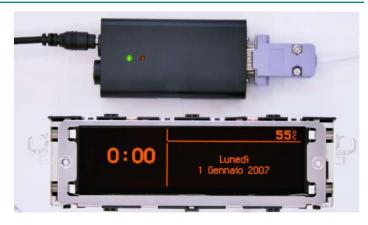
Switch on the module on a test bench using the Minitools CAN BUS generator SEP-CAN-INFO1, or directly on the vehicle.
