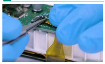
With the aid of tweezers, insert the FPC of the new display, with contacts facing down, into the connector on the small PCB.
