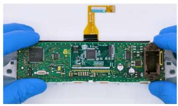
Peel off the rear protective film, fit the display into its housing and attach the PCB on the rear side of the module.
