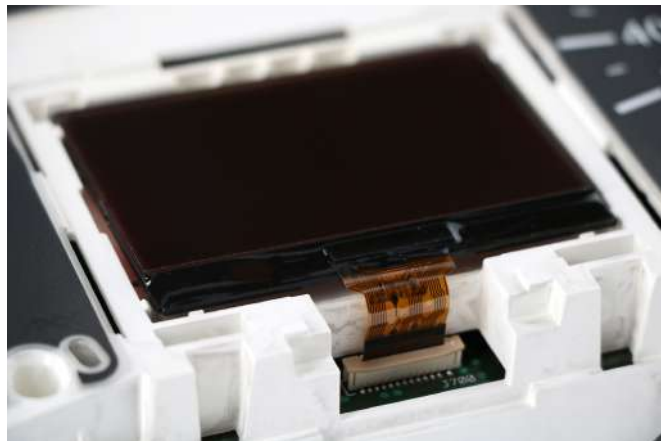
Carefully position the display in its plastic housing until it is in the correct position. Then secure the display in place with the metal frame.
