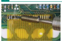
Solder the FPC pins on the board one at the time with a soldering iron with conical tip at 350°C.
