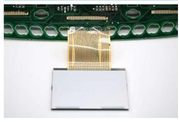
Detach the flat of the original display from the motherboard by simply pulling it away.
